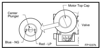
Fig. 63 Depress and turn center plunger.
